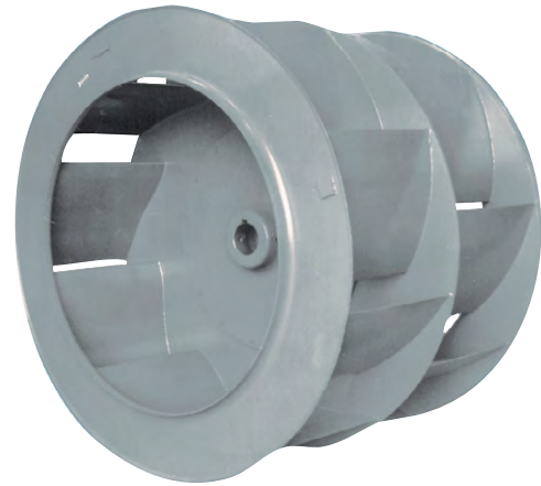
CAE-DW wheel with hollow airfoil blades staggered for improved sound quality
